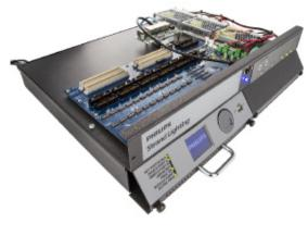
With a major performance upgrade for C21 dimmer racks, the new processor delivers a new level of connectivity to C21 systems. A new front panel design with integral Ethernet port, together with an integral 4 port ethernet switch makes connection simple. Two DMX512 inputs are standard with the second input available for use as an RS485 port supporting our Vision.net control system.
